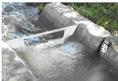
Fig. 1. Visual measurements of levels: а — a measuring scale on the surface of a concrete pillar in front of the groove; б — staff in a still niche in front of the trapezoidal spillway [2] (photo of the author)
