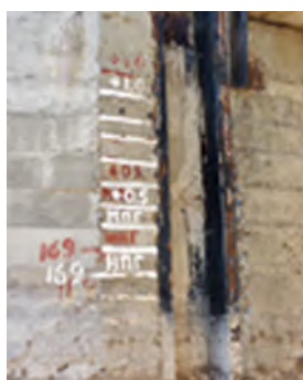
Fig. 1. Visual measurements of levels: а — a measuring scale on the surface of a concrete pillar in front of the groove; б — staff in a still niche in front of the trapezoidal spillway [2] (photo of the author)
