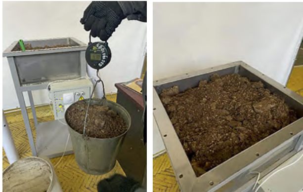
Fig. 2. Weighing of processed animal by-product and loading it into the chamber. Photo IEEP. St. Petersburg. 2024
