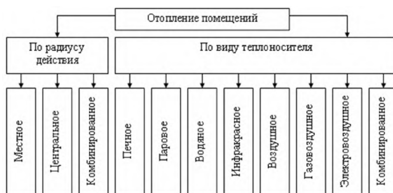
Fig. 1. Classification of heating systems
