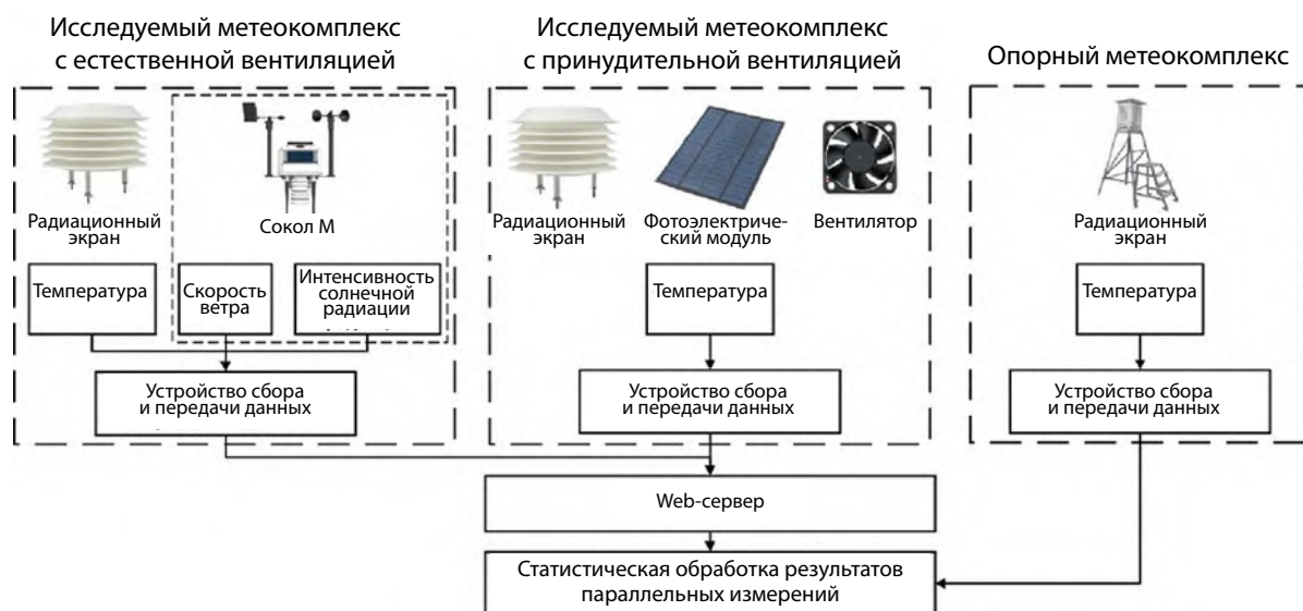
Fig. 2. Structural diagram of the experimental stand. The author's drawing
