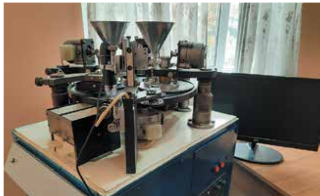
Fig. 2. A device with software and technology for dividing the grain of silkworm breeds labeled by sex
