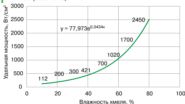
Fig. 2. Change in the power density of microwave energy losses during the dehydration of hop
