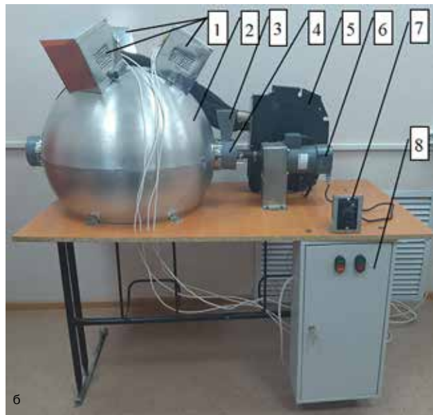
Fig. 1. Continuous operation microwave wax melter with semi-spherical resonators: а — schematic representation of the melting process; б — microwave wax melter (prototype); 1 — microwave generators; 2 — resonator chambers with an annular disk inside; 3 — receiving tank; 4 — injection screw in the casing; 5 — magnetron cooling fan; 6 — gear motor; 7 — frequency converter; 8 — control cabinet
