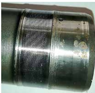
Fig. 3. The seat of the drive axis of the cylindrical straight tooth gear of the «John Deere» tractor with a «torn» thread
