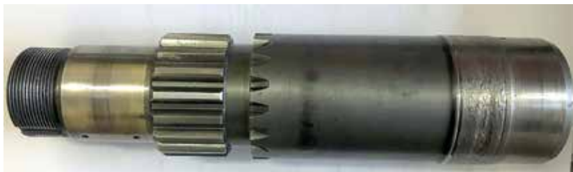
Fig. 1. The drive axis of the cylindrical straight tooth gear of the «John Deere» tractor with a worn-out seat
