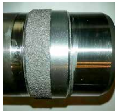
Fig. 4. The restored seat of the drive axis of the cylindrical straight tooth gear of the «John Deere» tractor
