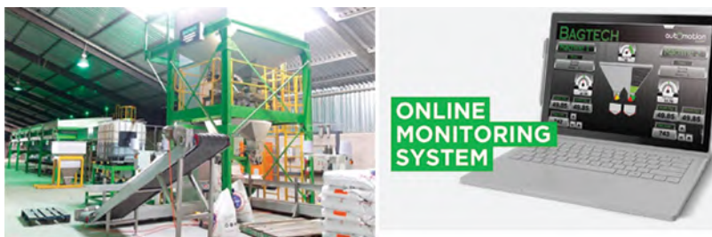
Fig. 15. Mixing plant and online monitoring system with real-time graphics 17
