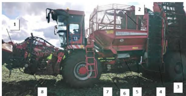
**Fig. 1.** General view of the Holmer Terra Dos T3 beet harvester equipped with a separation system with exhaust gas heat ("Krasnaya Gorka" LLC): 1 — topper; 2 — hopper; 3 — discharge conveyor; 4 — rod loading conveyor; 5 — deflector; 6 — air duct; 7 — separating stars; 8 — grubber
