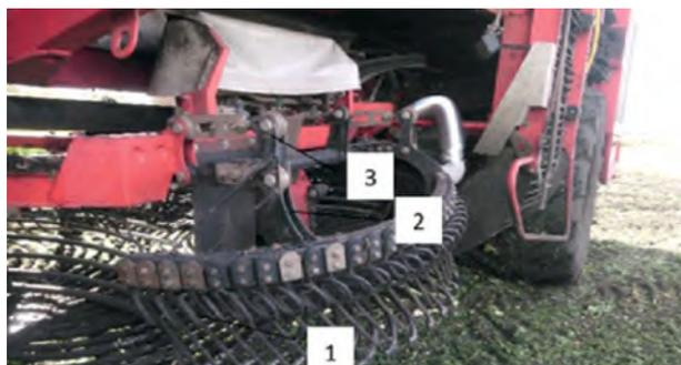
**Fig. 2.** General view of the separation system using the exhaust heat of the engine of the Holmer Terra Dos T3 beet harvester (Krasnaya Gorka LLC): 1 — separating star; 2 — deflector; 3 — air duct
